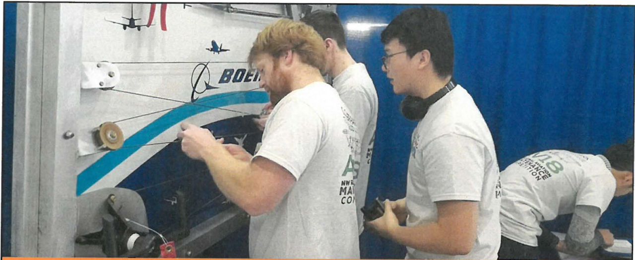
Cable Tension and Rigging mockup provided by the Boeing Company
